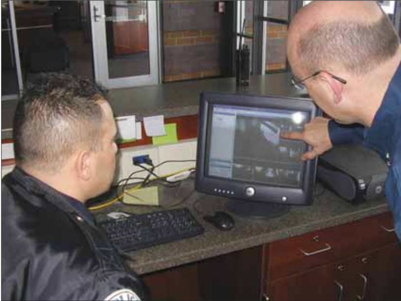
Greg Coons, service manager with ProTech Security of North Canton, Ohio, and J.J. Lenevier, safety officer with Jackson Township Police Department, discuss the different camera layouts and the possible views available using Milestone software. IP cameras that connect to the head-end using the school's LAN provide the video feed.
